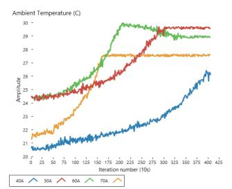
Regarding the discharge test with 4 different current rate, ambient temperature reaches the maximum value when Module is fully discharged and there is quite correlation between consumed energy and Module ambient temperature. Temperature increase window is 5 Celsius.
