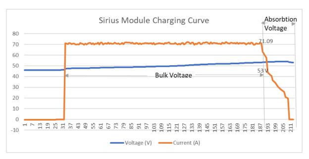
Figure 1:Sirius Module charging curve.
